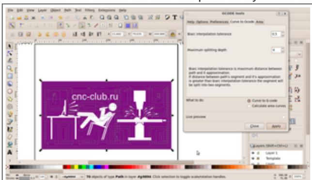
7. After applying Calculate area curves you should have a new group containing paths that cover the area of the
