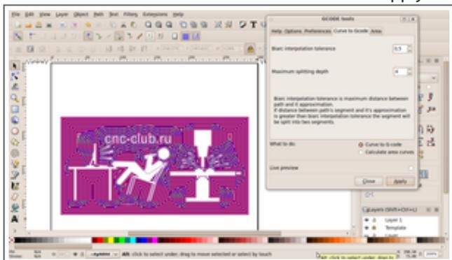
What you'll get: a group will be added to the drawing which shows cutter's working trajectory, and of cause a file in specified directory which will contain Gcode.
